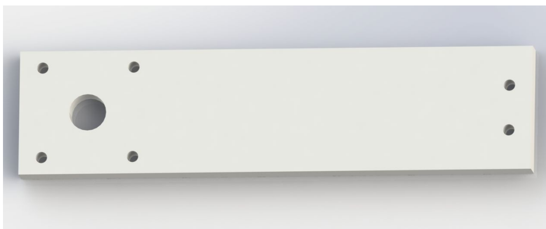
Figure 36: PVC baseplate Render
