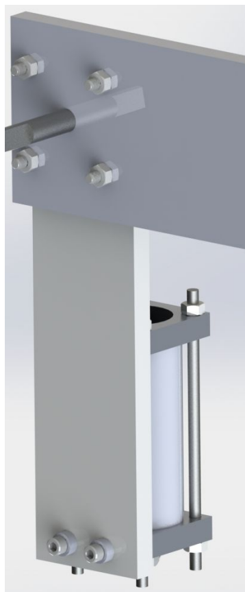
Figure 31: Back view of connection to provided faceplate and view of connection between PVC plate and endcap
